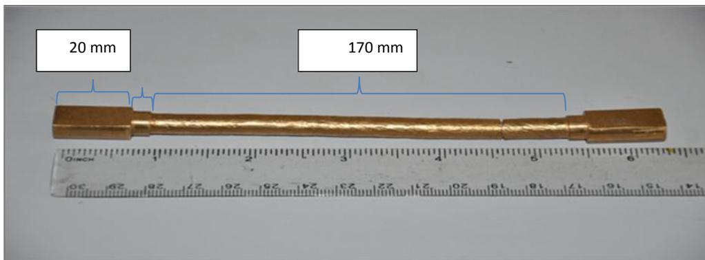
**Figure 2.** Metal Sample after torsion testing.
