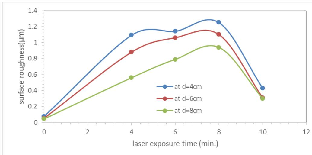
**Figure 5.** Surface roughness versus laser exposure time for 4 cm, 6cm and 8 cm distances from laser source.
