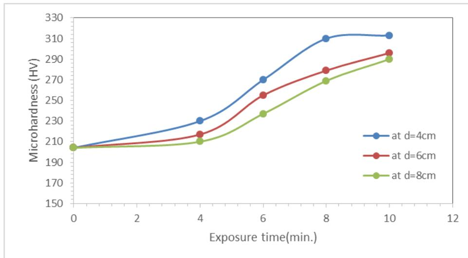
**Figure 6.** Micro hardness versus laser exposure time of 4 cm, 6 cm and 8 cm of distance from laser source.
